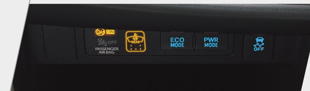
ECO & POWER Drive Modes | ECO mode for optimum fuel economy and POWER mode for sharper acceleration response
